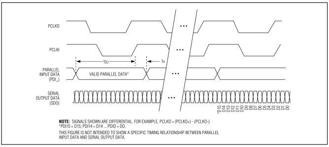
Figure 4. Parallel and Serial Data Timing
